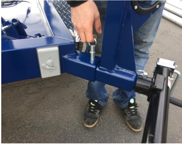
Figure 3. Slide the Jack Extension Tube Out
