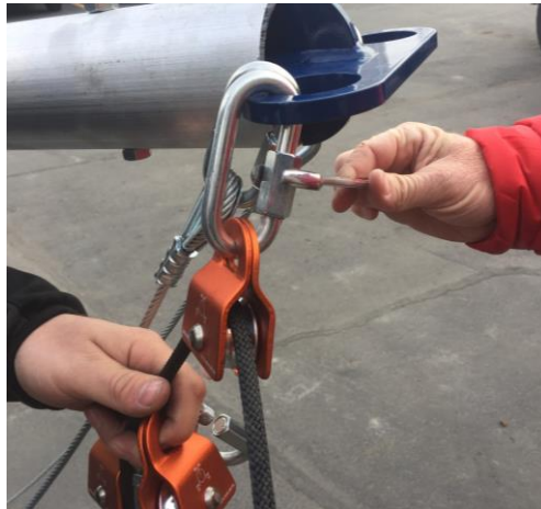
Figure 14. Attach Rope, Quick Link, and Pulley to Pole.
