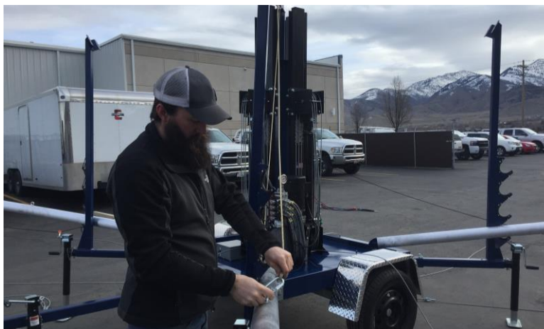
Figure 25. Connecting the Winch Rope to the Lift Point on the Pole
