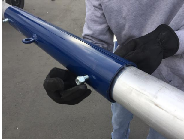
Figure 9. Upper Section Slides into Sleeve of Lower Section
