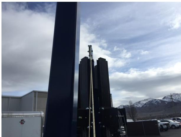
Figure 24. Winch Rope Routed Over the Removable Directional Pulley
