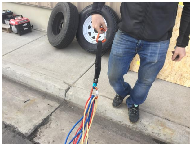
Figure 20. Use a Girth-Hitch to Attach the Lanyard to the Swivel
