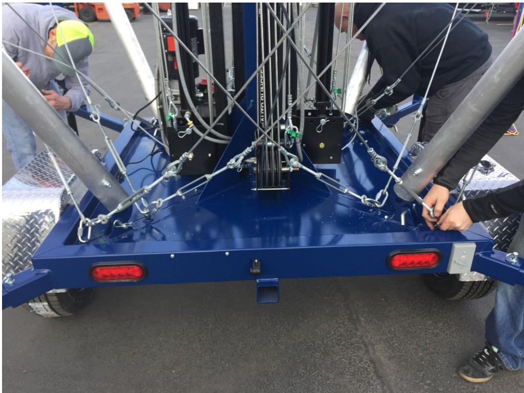
Figure 32. Tighten Quick Links and Tension Turnbuckles.
